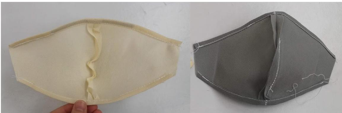
*Figure 4: Shell fabric with aluminium nose piece inserted (left), lining fabric (right)*
