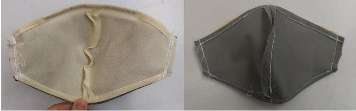
*Figure 6: Shell and lining fabric sewn together along edges*
