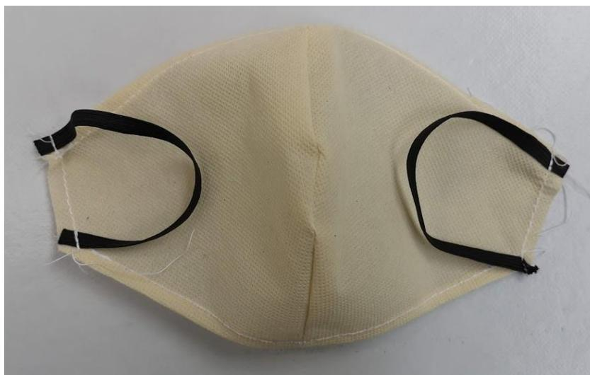
*Figure 5: Shell fabric with elastic ear straps attached*
